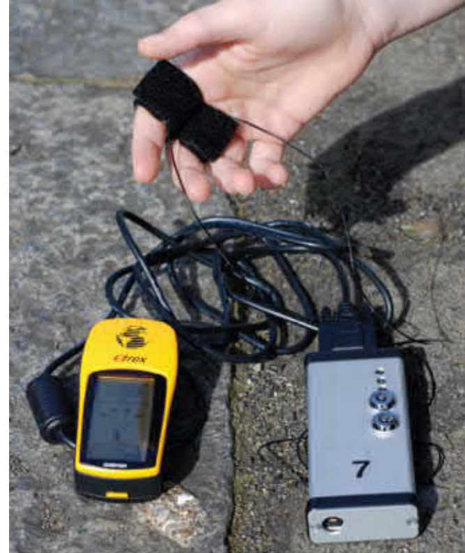
The Bio Mapping device: GPS - left, fingerclip - top and data logger on the right.
